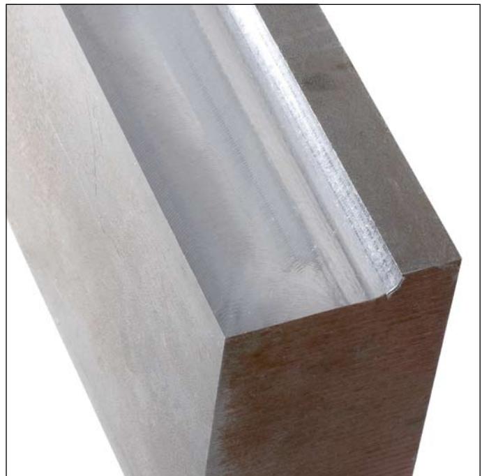
Part milled with ACC: At the same feed rate and cutting depths the surface shows no chatter marks. The machining process took place with reduced loads on the tool and machine.
