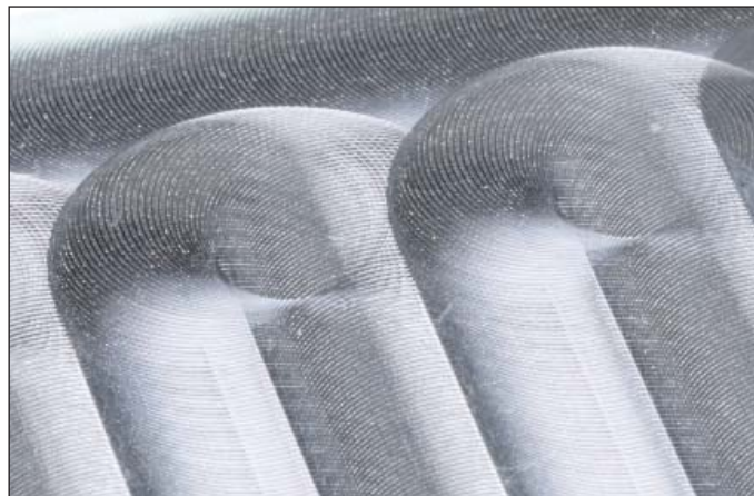
Figure 7: Machining without CTC
