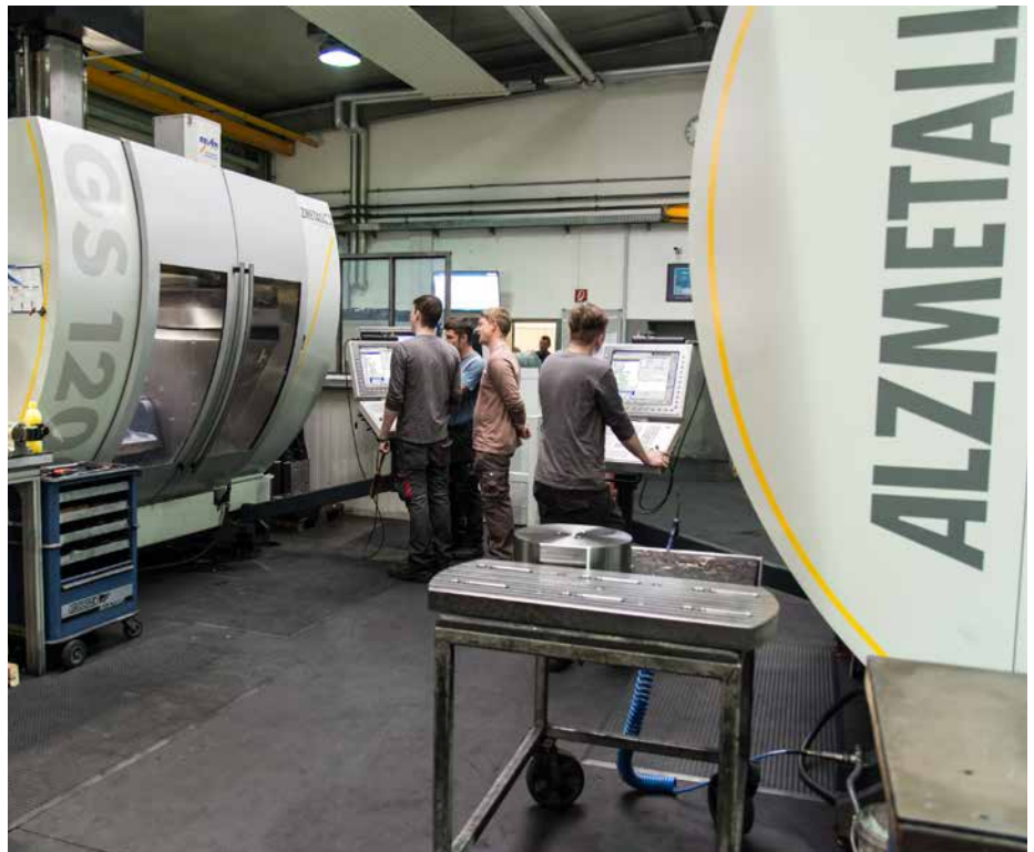
“Here we saw milling and turning working in unison.” The two new Alzmetall GS 1200/5 FDT machining centers with the HEIDENHAIN TNC 640.
