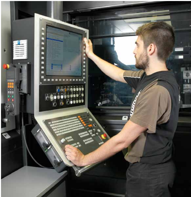
The machine operator can intervene manually during machining via the TNC controls.
