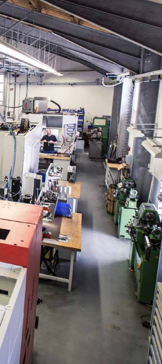
The production floor at WB mechanics: six milling machines with HEIDENHAIN controls, along with six lathes, are all connected to StateMonitor.
